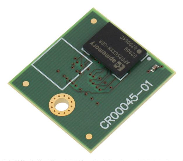
PSRAM add-on board for AP Memroy PSRAM devices, 8 and 16 bit mode supported. VCCIO adjustable must be 1.8V.
