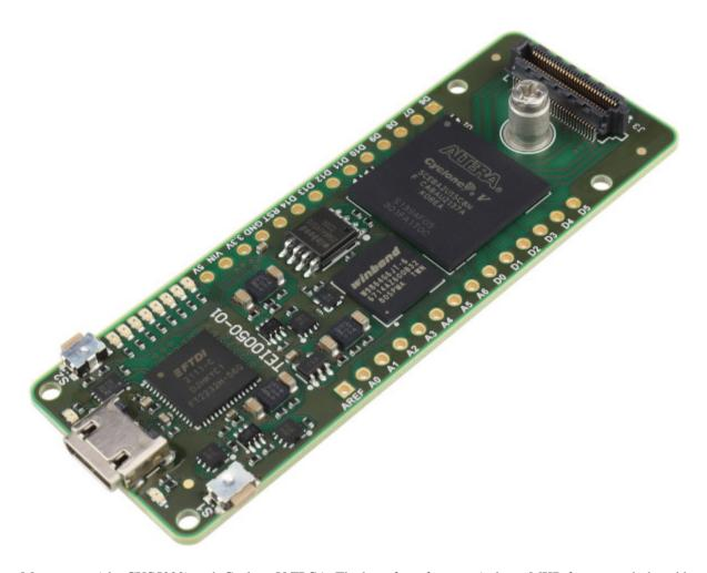
Mini carrier (aka CYC5000) with Cyclone V FPGA. The base form factor is Arduino MKR format, with the addition of one CRUVI HS connector at the edge.
