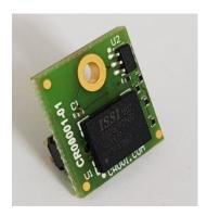
This module is a simple SPI Flash add-on board. Can be assembled with any SPI flash in BGA24 6x8 mm package. I2C identification EEPROM is provided. Note that only 3.3V SPI Flashes are supported by the standard CRUVI LS hosts. It is allowed to use CR00001 with 1.8V Flash if your CRUVI LS host board supports 1.8V VCC for the LS slot.
