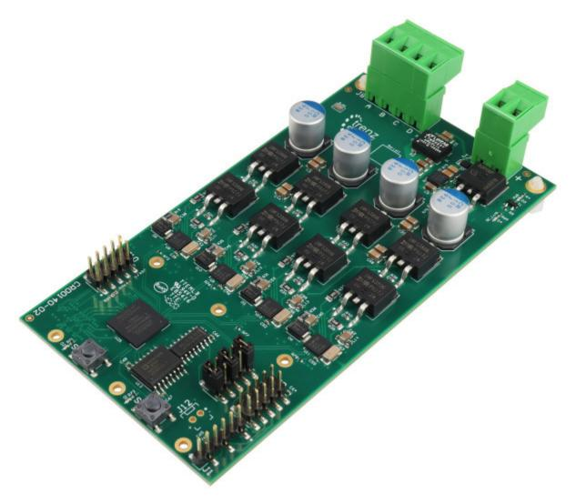
CRUVI HS board for motor control application. Tripple wide HS board with extended length.
